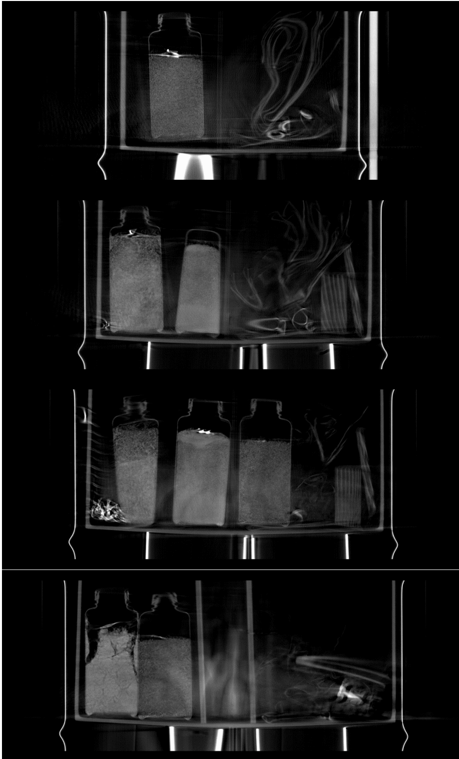
Figure 11 – 4 Vertical slices through 3D cone-beam volumetric data showing (from top to bottom): Dry Organic, Wet 50/50 & Wet Organic, Wet 50/50 & Wet Organic & Dry 50/50 and Wet Inorganic & Dry Inorganic.
