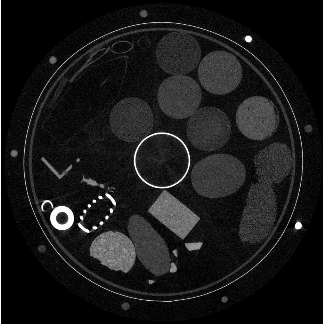
Figure 8 – CT slice from LDA based scanning with Copper and Tungsten in the set of rods
