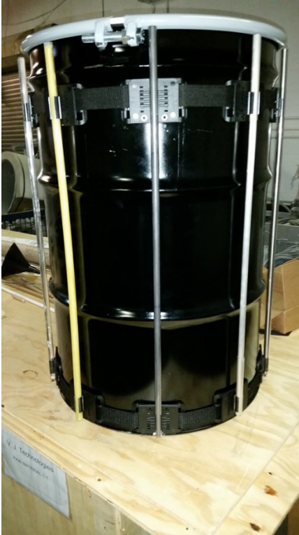
Figure 6 – Calibration jacket and rods attached to the outside of the Training Drum
